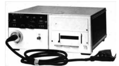
Figure 3: Hewlett Packard multi-wavelength ear oximeter.
