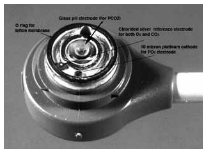
Figure 7: Combined PO 2 PCO 2 electrodes.
